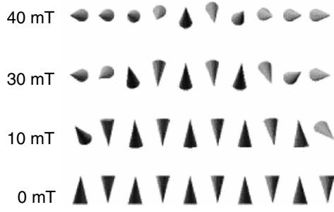
Figure 4. Spin configuration for the 550 nm diameter structures at selected fields, with the field applied out of the page. At 0 mT, neighbouring discs align anti-parallel. Increasing the field, the outer spins are the first to align as they are most weakly coupled.
